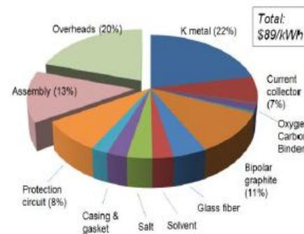
Figure 1: Cost breakdown of 1 kWh battery
